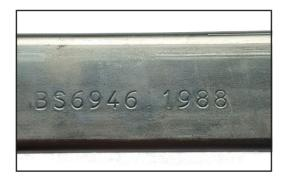
The engraving should also be clearly visible at all times, even when the product has under gone further finishing treatments i.e. Hot Dip Galvanised, Epoxy Coating. Contractors and distributors should be aware of cheap imported and non-standard products that have removable or no product marking at all, as this is not within the Standard.
